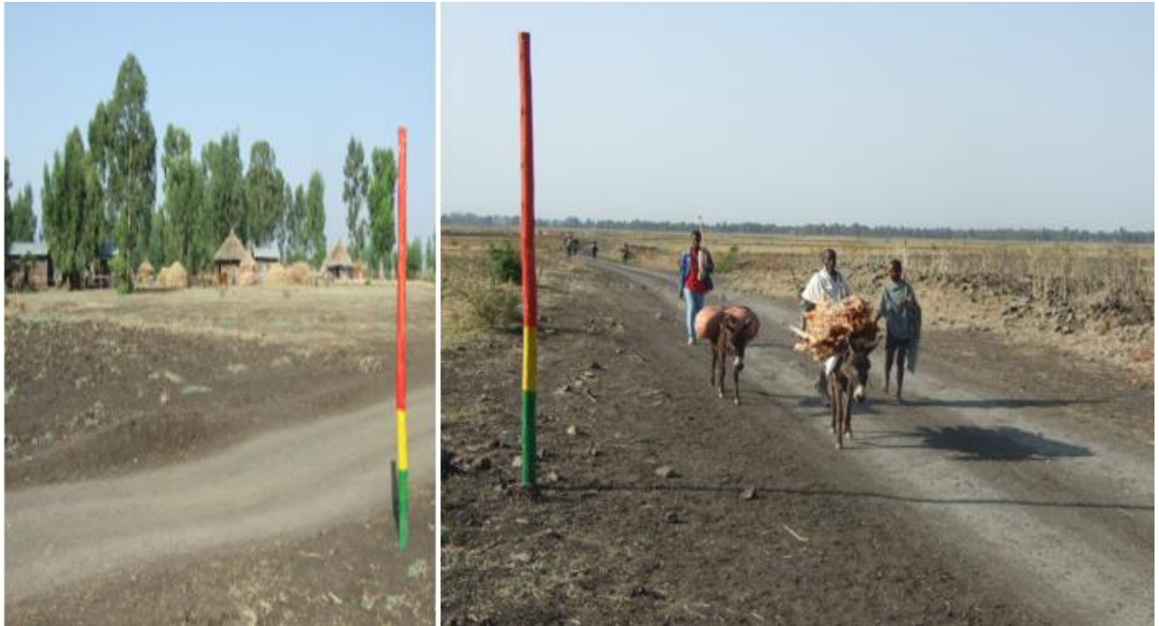
Figure 1.1 Manual Water Level Monitoring Pole in the Study Area
