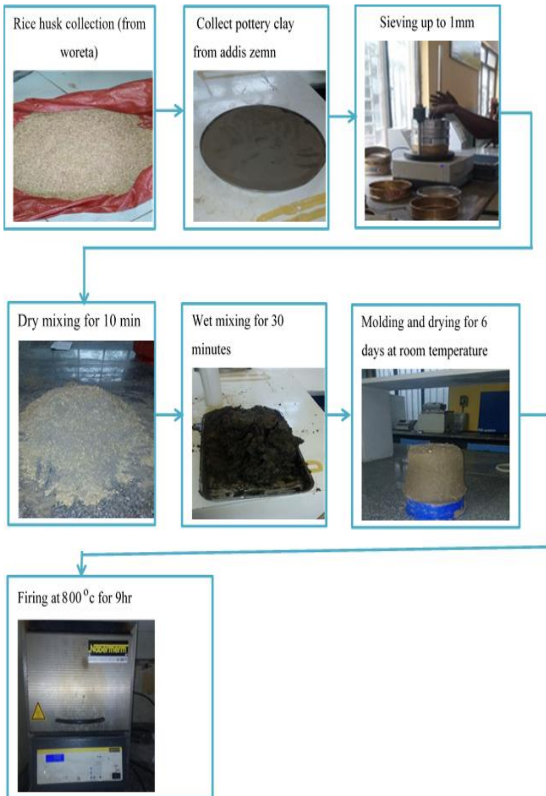
Figure 3.4. Preparation procedure of ceramic filter
