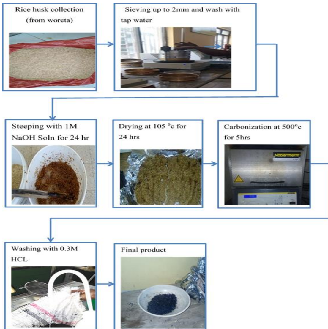
Figure 3.3. Preparation procedure of activated carbon filter
