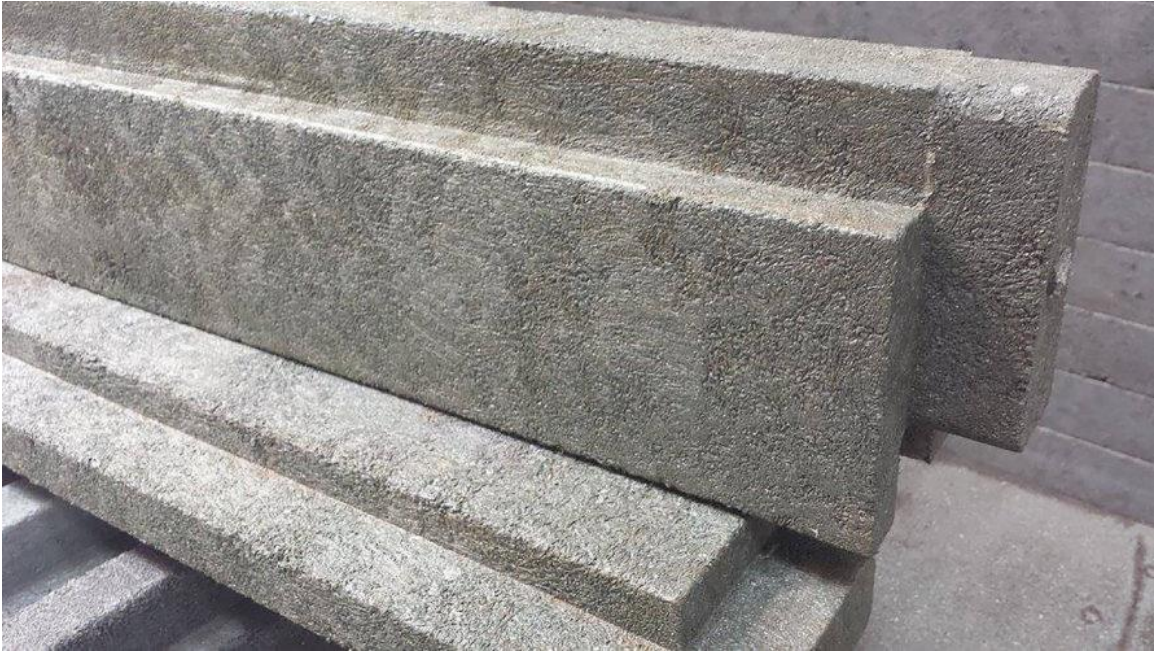
Fig 1. Sample bricks made by plastic wastes with sand mixture
