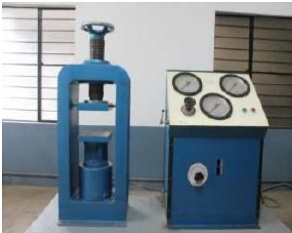
Fig 3HYDRAULIC TESTING MACHINES
