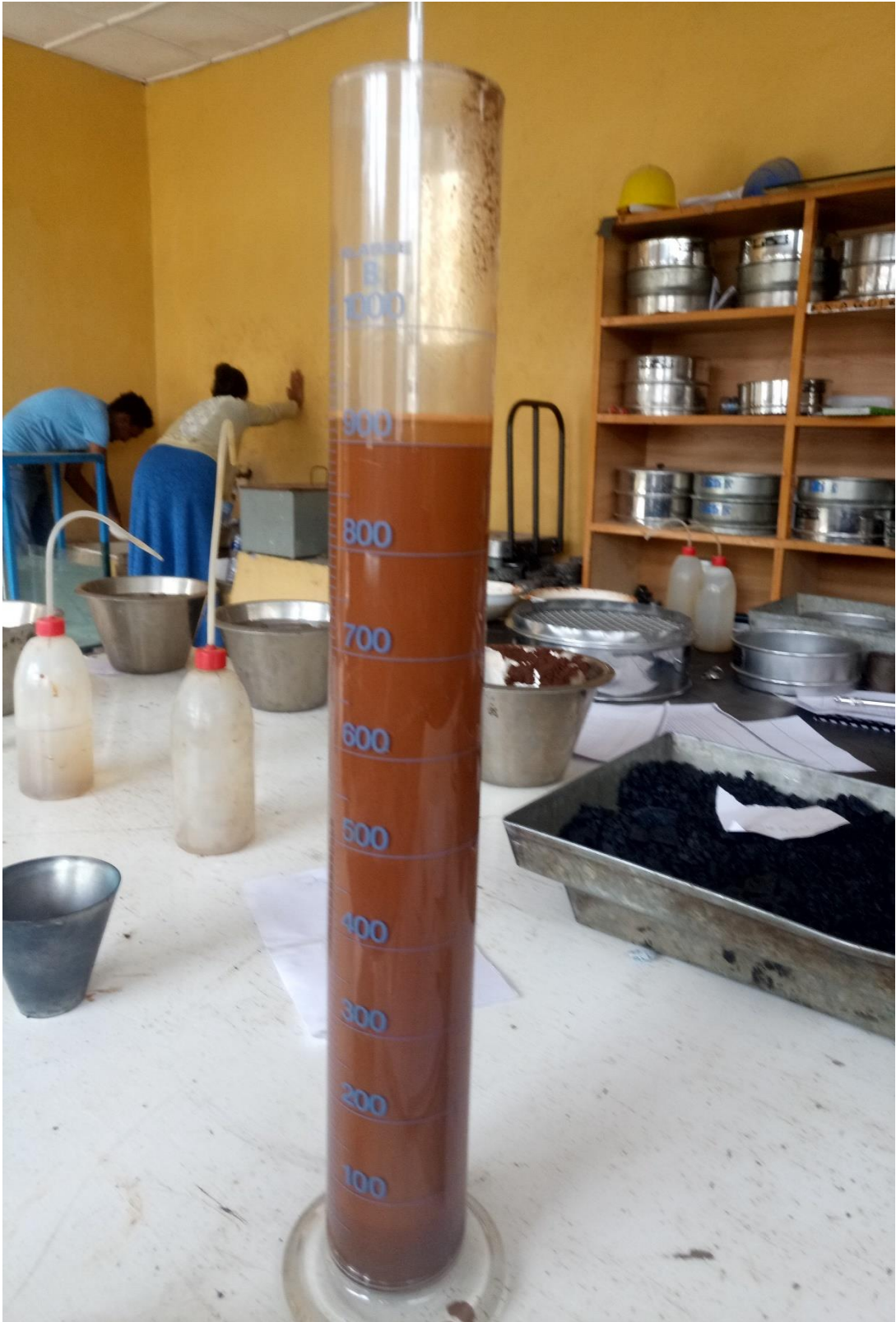
C-2, Grain Size Analysis (Hydrometer Analysis)
