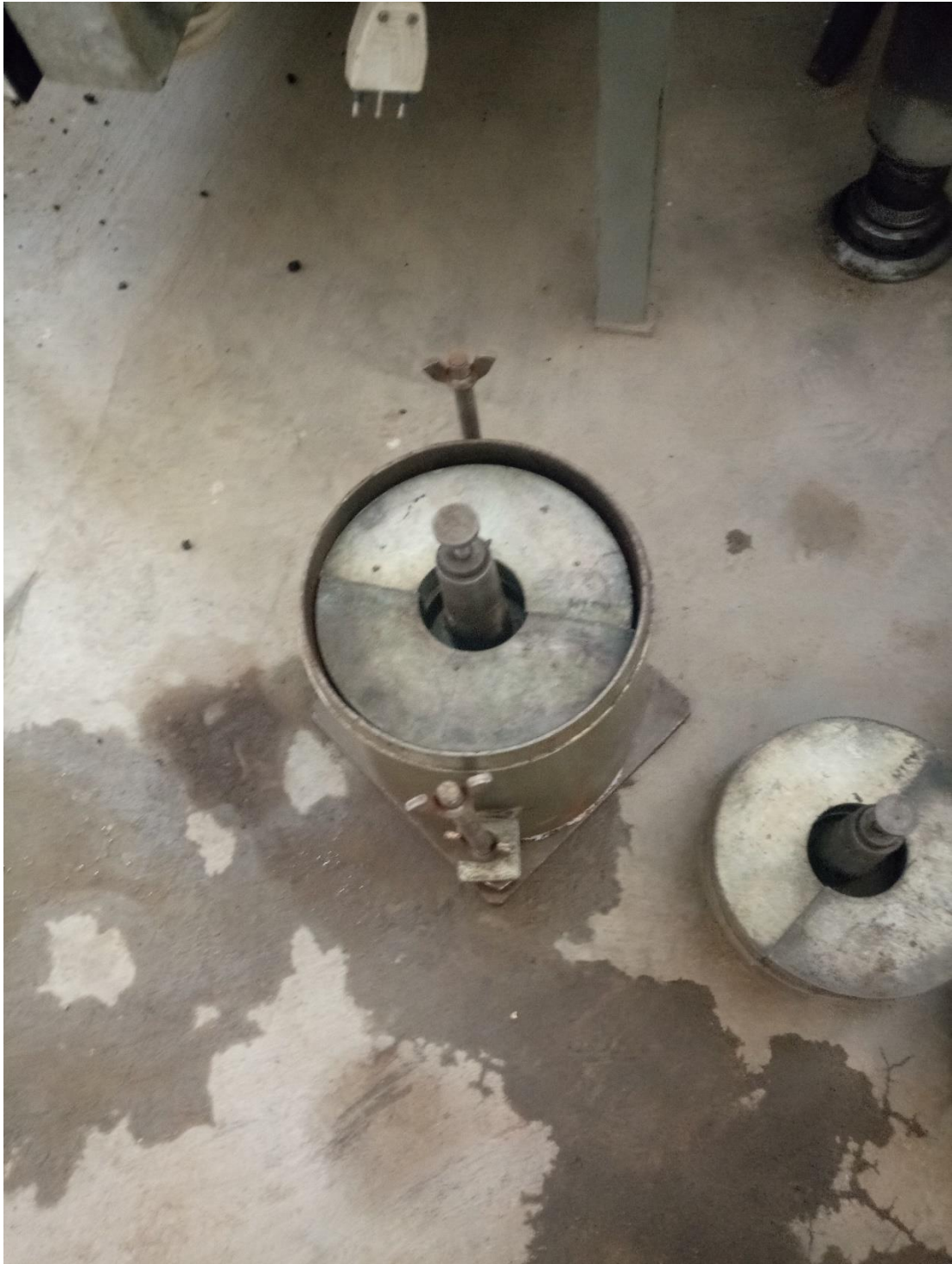
C-7, Compacted specimen with porous disks (before soaking)
