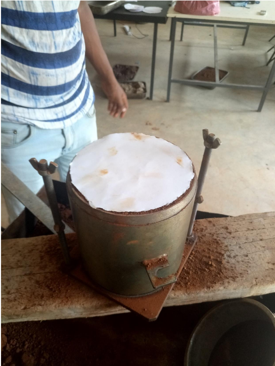
C-6, Compaction for CBR testing (using CBR mould)
