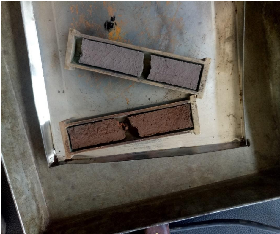
C-5, Linear Shrinkage Determination (Specimen after oven drying)
