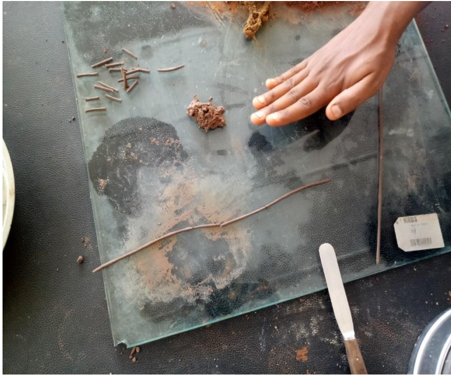
C-4, Plastic Limit Determination
