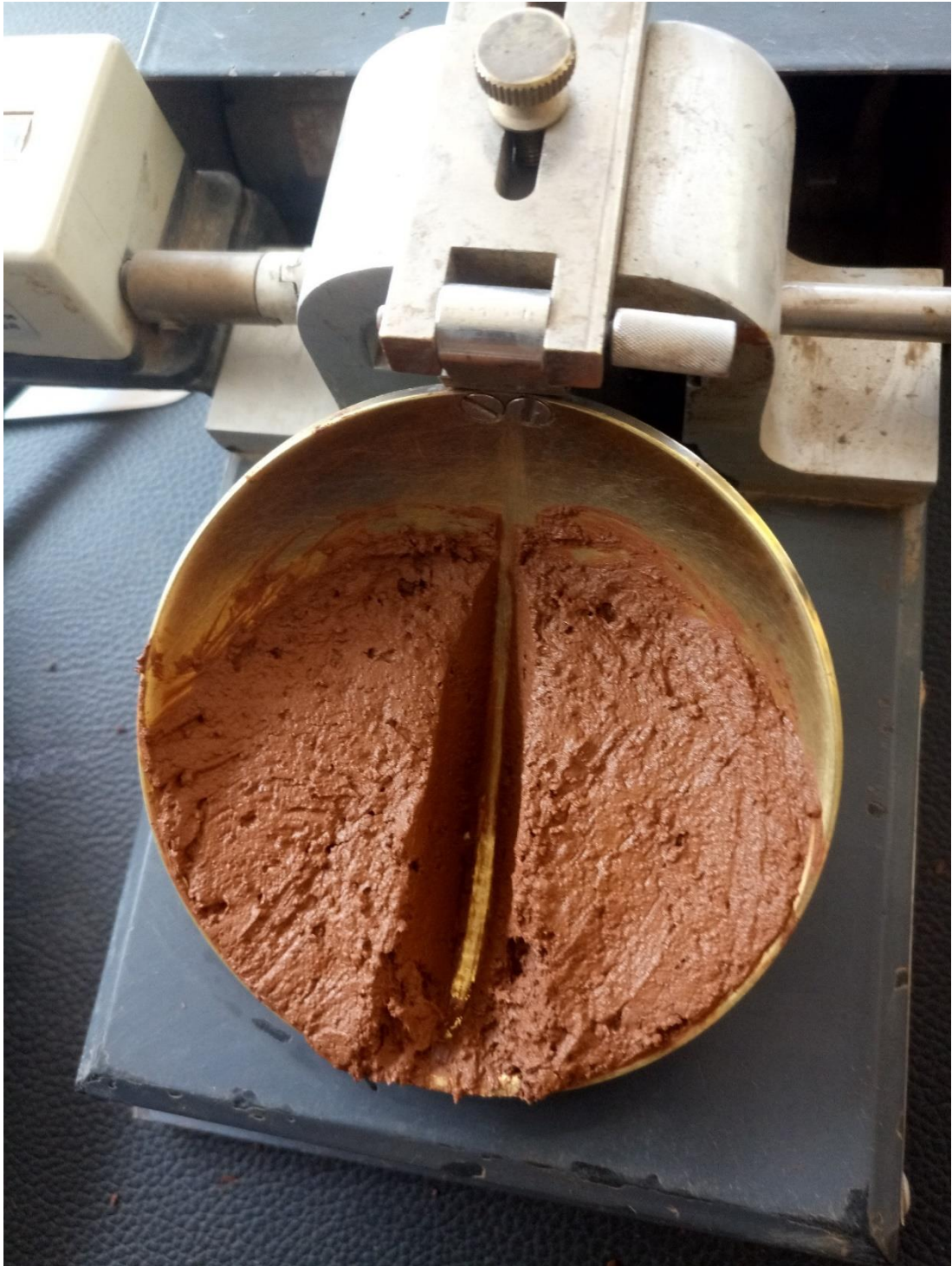
C-3, Liquid Limit Determination (Sample on Casagrande Cup)
