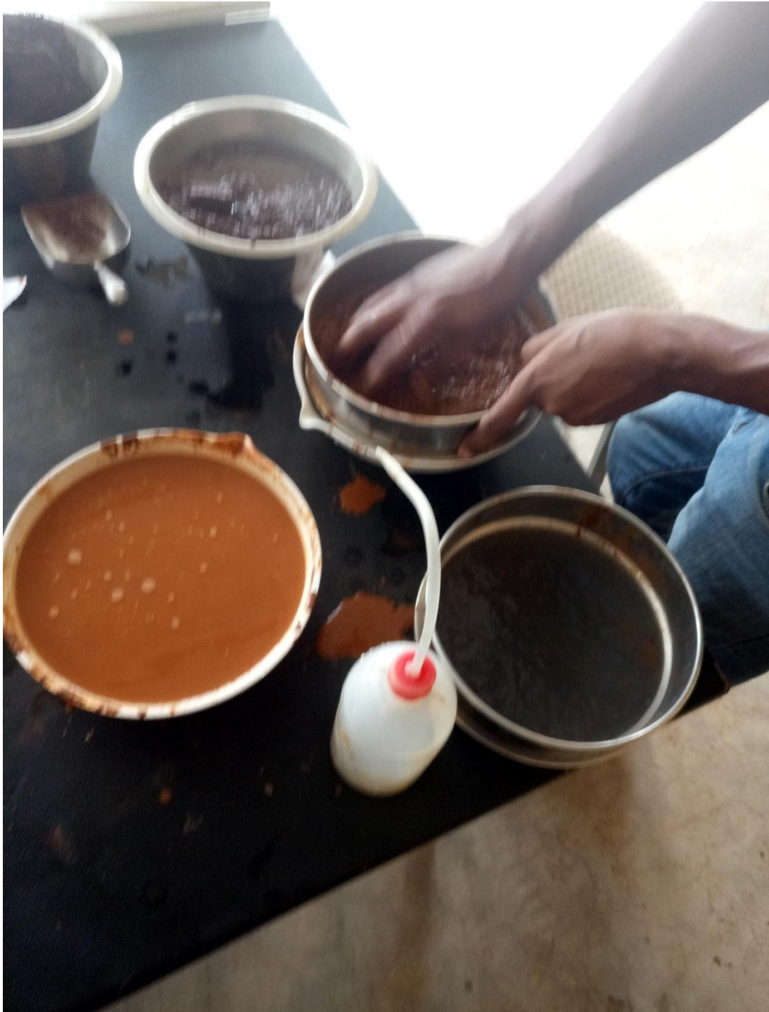
C-1, Grain size analysis (wet sieving)
